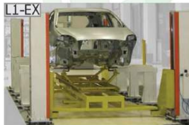
L1-EX Automatic system for in line controls on measuring robots
